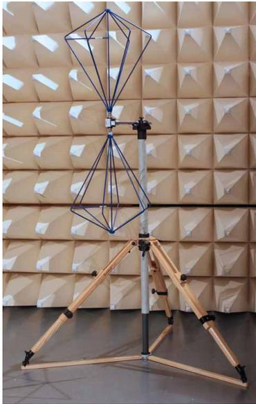
VBA 6106A vertical onto tripod
